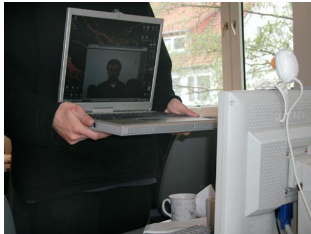
Figure 5: A face recognition is fooled by presenting the camera a simple picture of an authorised user on a laptop. [TKZ02]
