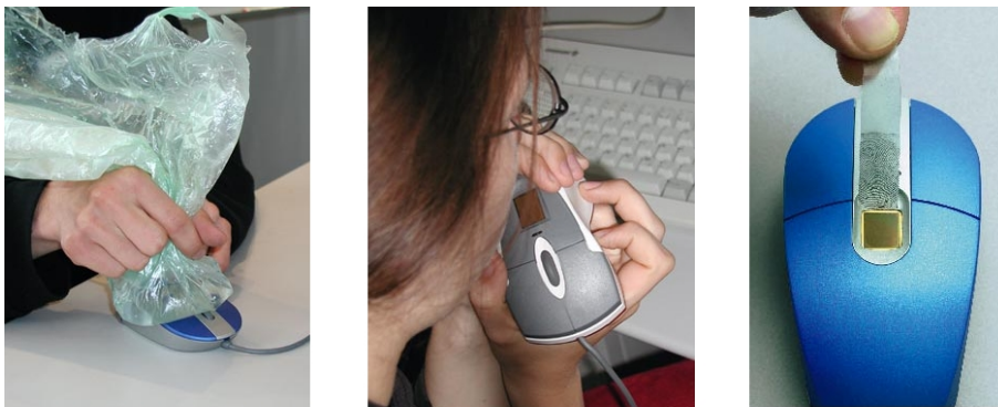
Figure 4: The three pictures from the article [TKZ02] show three different methods how it is possible to fool a fingerprint scanner.
